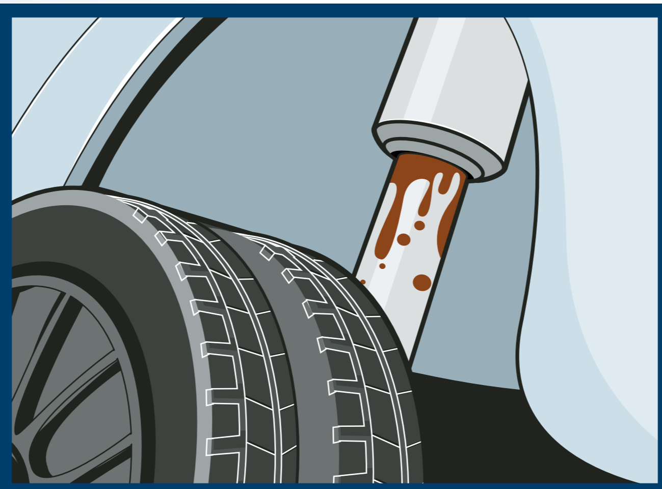
Oil on the shock absorber (a fine film of oil is needed for self-lubrication of the piston rod)
